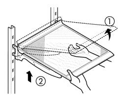
**To reinstall a shelf**—Tilt the front of the shelf up and guide the shelf hooks into the slots at a desired height. Then, lower the front of the shelf so that the hooks drop into the slots.
